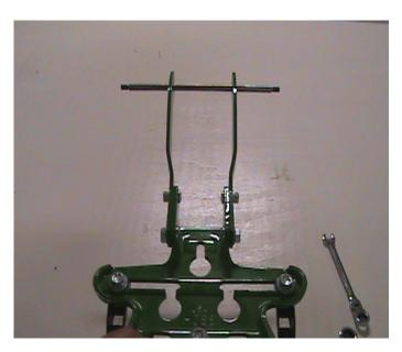
Step 4 Insert the axle shaft through the wheel mounting arms.
