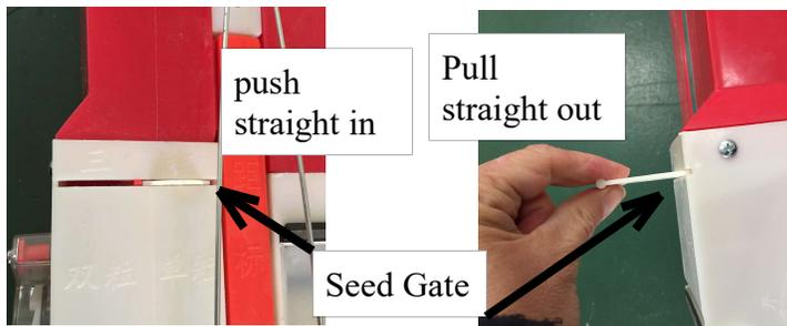
1. Push gate from back of planter to release it. Then pull gate straight out from front of planter.
