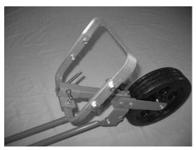
Flip the unit upside down, so the long hitch bar portion of the Frame is pointing upwards. This is the safest and easiest position for changing attachments. Fasten your attachment to the hitch bar using the Hitch Pin and clip.
