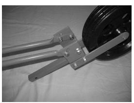
Using the 4 short bolts, connect the flattened ends of the lower Handle to the INSIDE of the Frame. The bolts that pass through the slots should be positioned in the middle of the slot.
