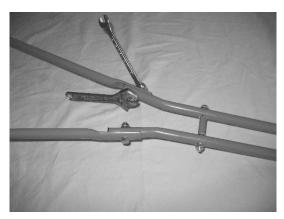
Using the other 2 long Bolts, connect the "V" end of the lower Handle to the upper Handles. Snug them, but do NOT tighten the bolts yet.
