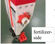
The side with the clear cover is the seed side. The side with the orange gear is the fertilizer side.
