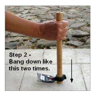
Step 2 Bang the flared end of the handle straight down against a solid surface TWO times to tighten it up.
