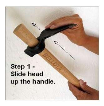
**Step 1 -** Slide the wood handle through the tool's eye until it fits snugly on the flared end of the handle.
