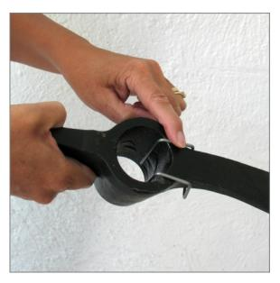
Push the two long wire ends down into the eye of the tool head.
