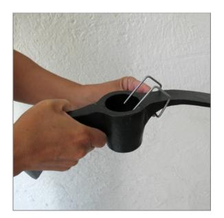
The retainer wire prevents the head from rotating on the handle.
